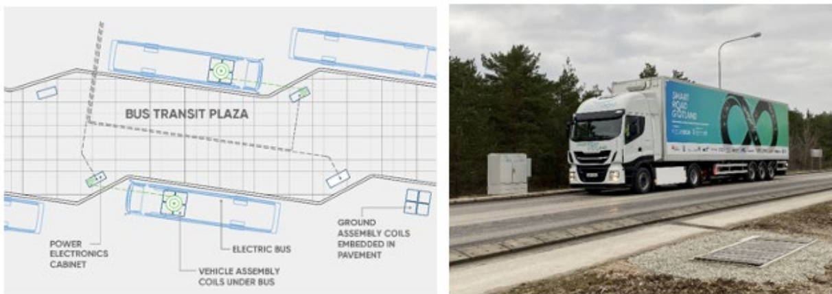
Figure 12: In-Road Inductive Charging and Static Inductive Charging (Sources: ElectReon and Momentum Dynamics)
