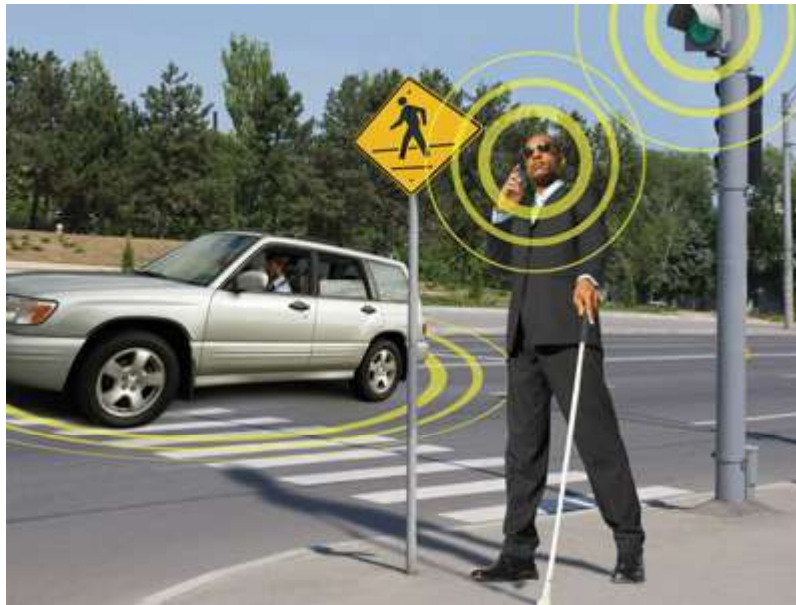
Figure 16. Information about this blind pedestrian's location is broadcast to approaching vehicles (Source: Intelligent Transportation Systems Joint Program Office)
