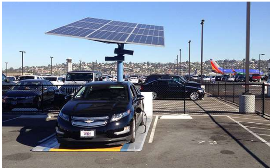
Figure 12. Chevy Volt plugged in to a renewable, portable charging station.
