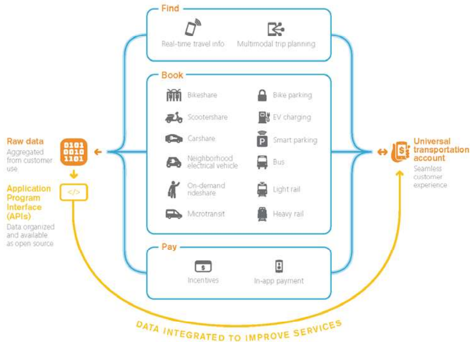
Figure 3. Mobility as a Service provides an integrated platform for trip planning and booking across modes
