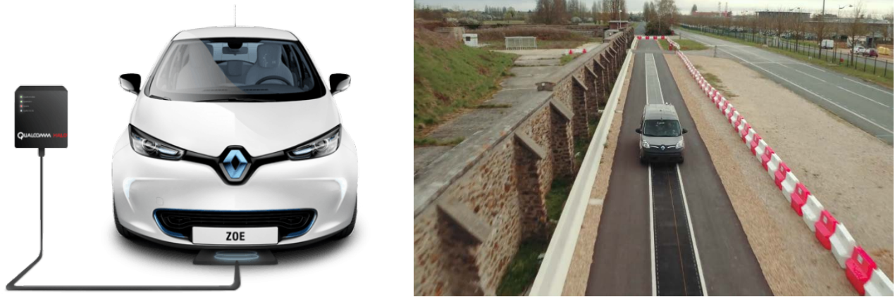
Figure 11. Static and in road Inductive Charging (Source: QUALCOMM)
